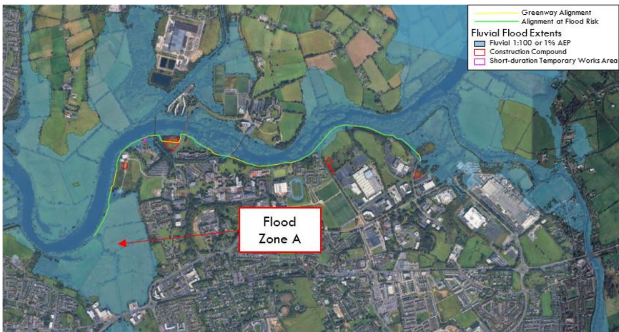
Figure 3-138: Sections of Greenway at Flood Risk (1 in 100 or 1% AEP)
